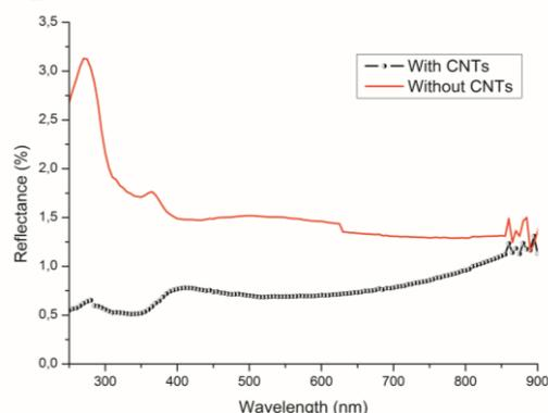
Figure 1 Reflectance measurements on samples with and without CNTs
